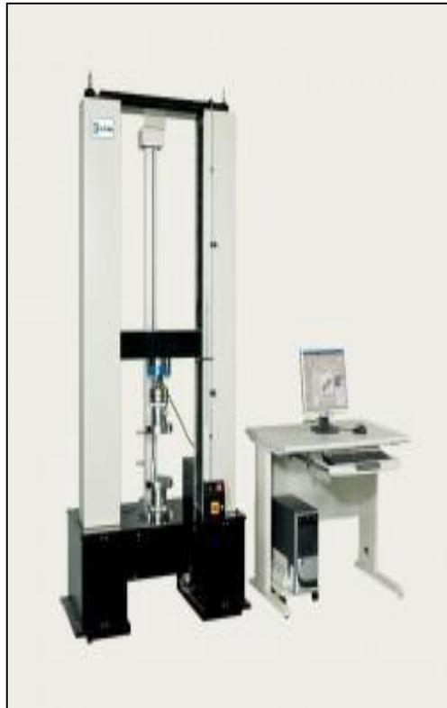
**Gambar 1.9** Tensile Machine
