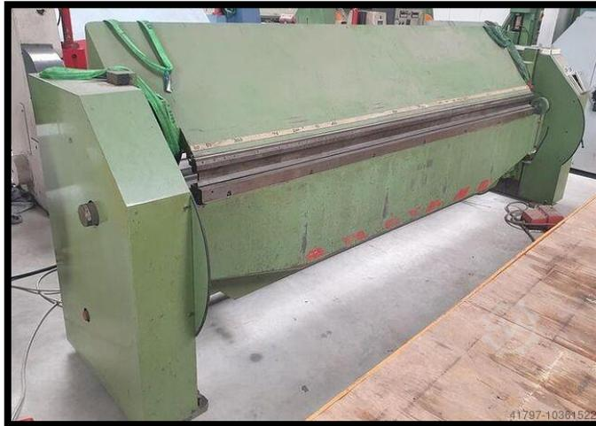
**Gambar 2.3** Alat bending
