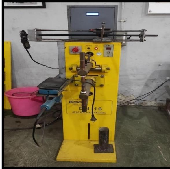
**Gambar 2.2** Resistance spot welding
