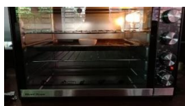
Sampel dioven ( T=100^\circ\text{C} , t=2 jam)
