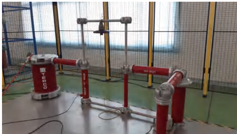
(Rangkaian Percobaan Pengukuran Flashover / Withstand Test )
