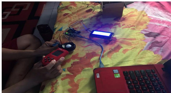
Gambar 32. Kalibrasi sensor BH1750
