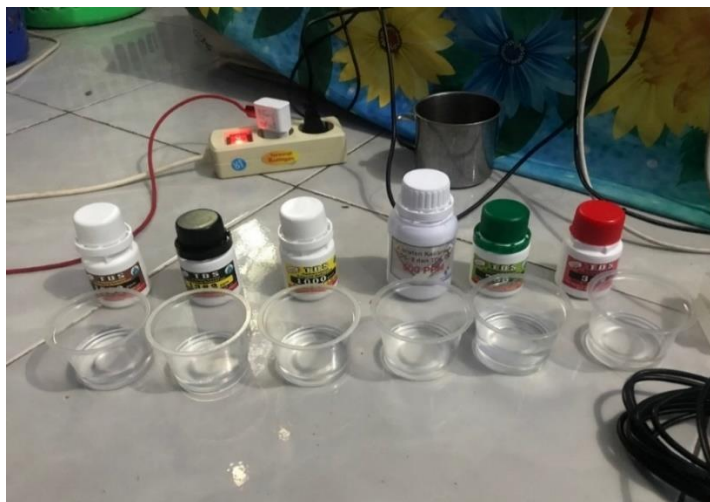
Gambar 33. Kalibrasi sensor TDS
