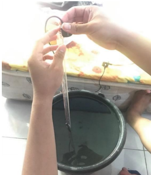
Gambar 34. Kalibrasi sensor JSN-SR04T
