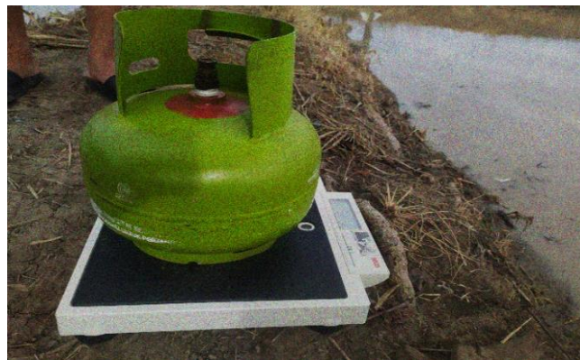
Gambar 7. Penimbangan gas LPG
