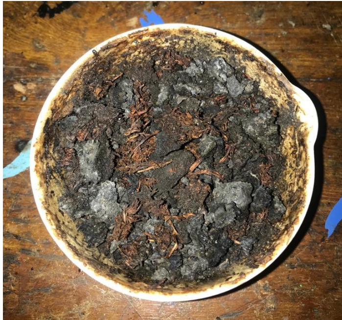
Gambar L4- 12. Biochar ampas sagu setelah pretreatment perendaman NaOH 10% dan microwave pyrolysis 540 watt
