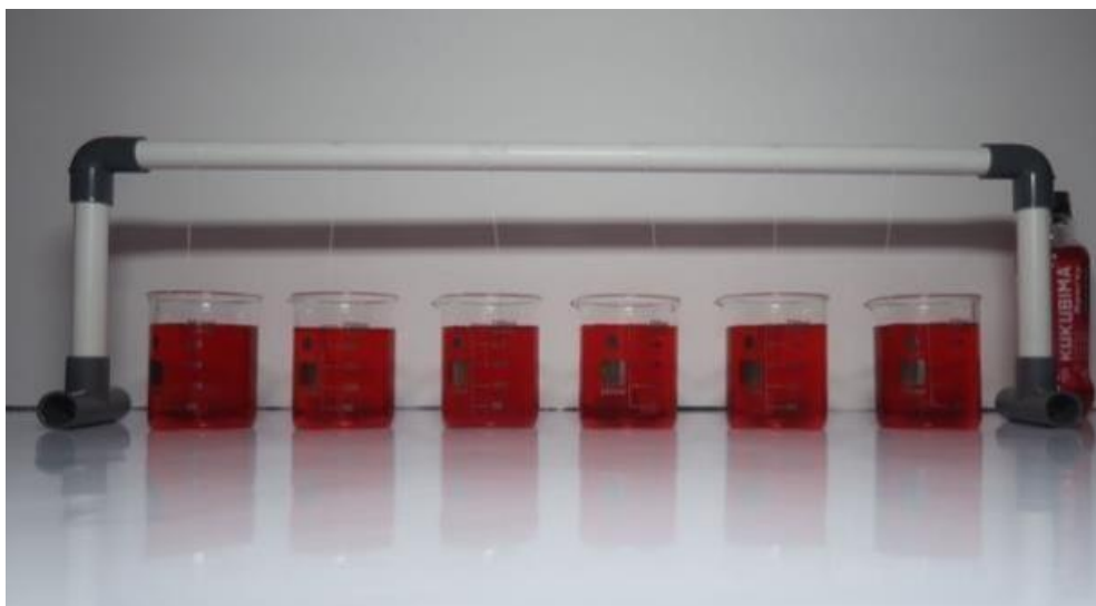
Immersion of thermoplastic nylon resin in Kukubima energy drink
