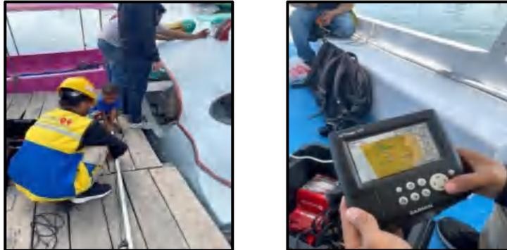
**Gambar 8.** Pengukuran Survey Batimetri *Ecosounder*
