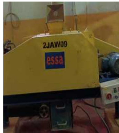
Jaw Crusher -20 mm, -10 mm, dan Roll Mill -3 mm
