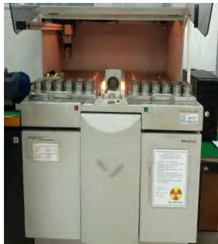
X-Ray Fluorescence Spectrometry (MagiX Fast)
