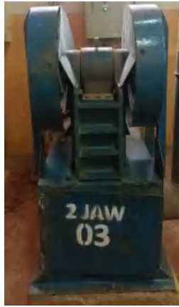
Jaw Crusher -20 mm, -10 mm, dan Roll Mill -3 mm
