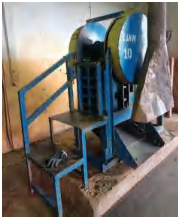
Jaw Crusher -20 mm, -10 mm, dan Roll Mill -3 mm
