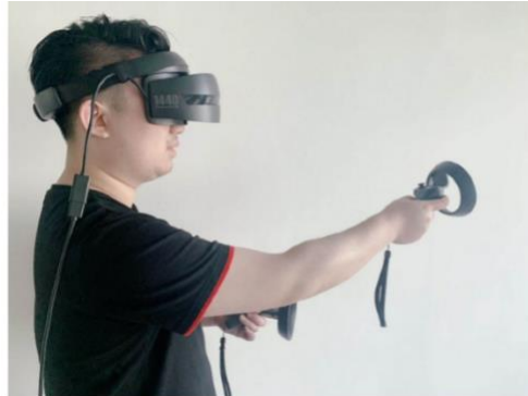
(Figure 1) Head-mounted display and gesture sensor ( li Y. et al. 2021. The Current Situation and Future Prospects of Simulators in Dental Education )
