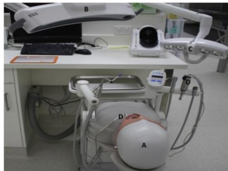
(Figure 2) The components of the DentSim (A) Phantom Head, (B) Overhead Infrared Camera, (C) Light Source, (D) Infrared Sensor. (Roy et al. 2017. The need for virtual reality simulators in dental education: A review )
