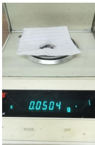
Gambar 6. (a) Proses Penimbangan Adsorben Magnetit (b) Optimasi pH Optimum Larutan Ion Logam Cd(II)
