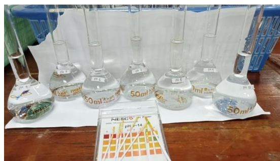
Gambar 6. (a) Proses Penimbangan Adsorben Magnetit (b) Optimasi pH Optimum Larutan Ion Logam Cd(II)
