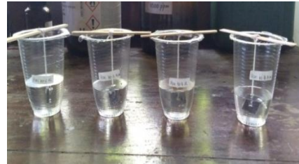
12. Proses perendaman baja tanpa inhibitor
