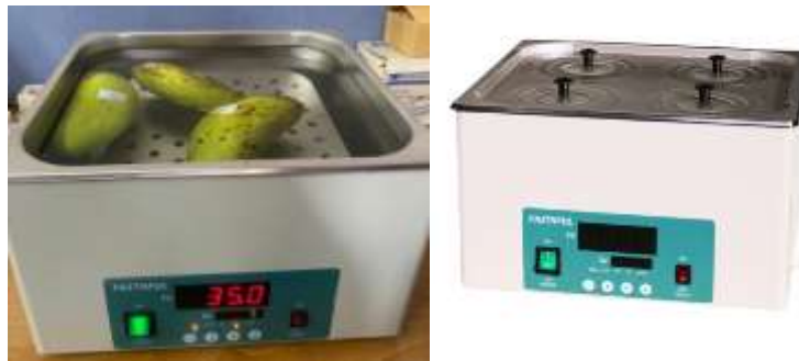
Gambar 4. Hot Water Treatment
