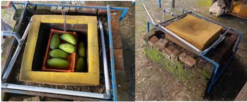
Gambar 2. Zero energy cool chamber (ZECC)
