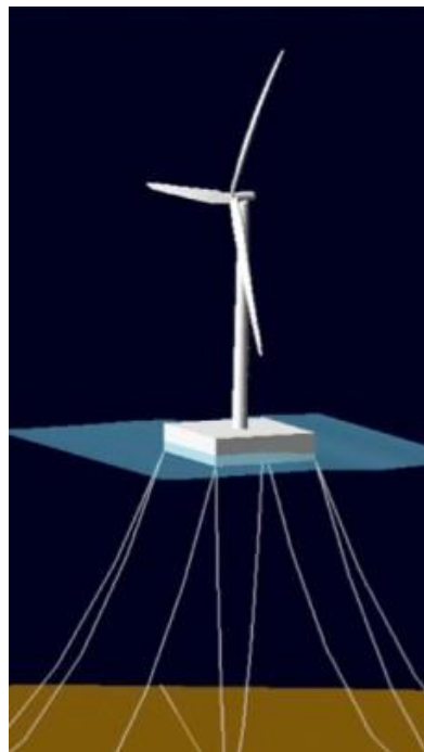
Gambar 2 Platform dan tower turbin terapung ITI Energy Barge
