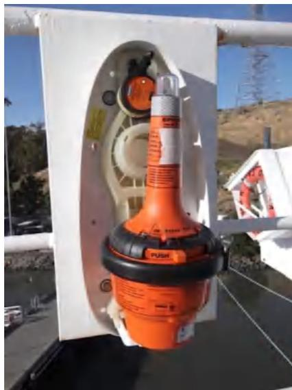
Gambar 11 *Emergency Position Indicating Radio Beacon (EPIRB)*
