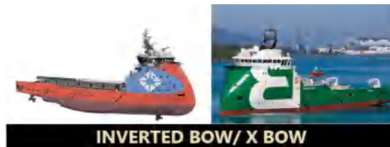
Gambar 12. Haluan kapal inverted bow
