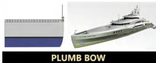
Gambar 5. Haluan kapal plumb bow/straight bow
