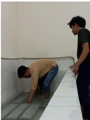
Perawatan wet curing balok
