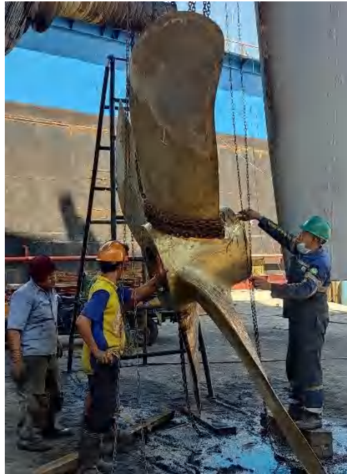
Gambar 11. Perawatan propeller kapal: proses polishing
