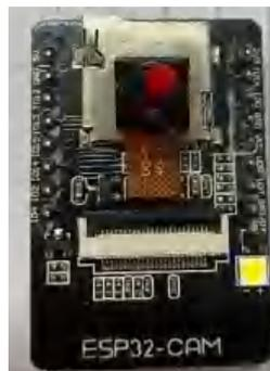
**Gambar 3** Modul ESP 32 CAM
