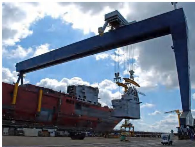
Gambar 18 Gantry crane (sumber: Kino Cranes)
