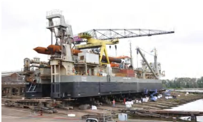
Gambar 7 Slipway jenis side launching (sumber: Wikimedia Commons)
