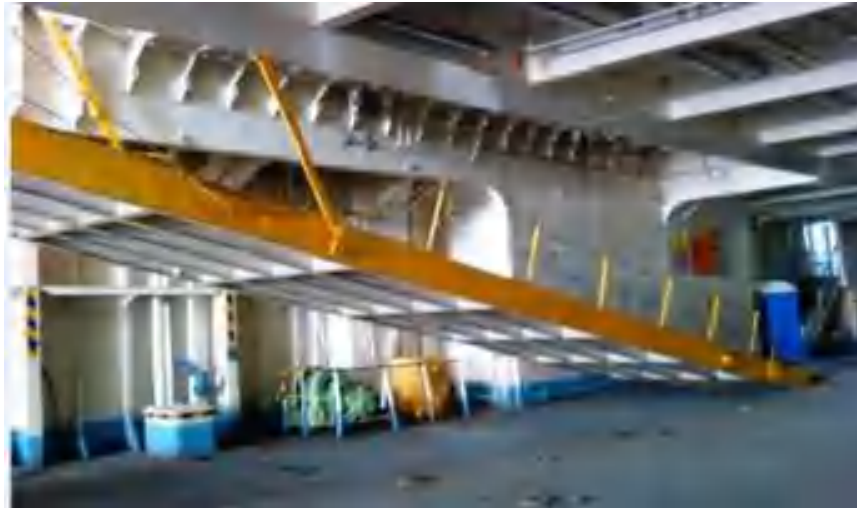
Gambar 2. Ramp Door internal KM Dharma Kencana VIII (Sumber: Kristyson, 2014).
