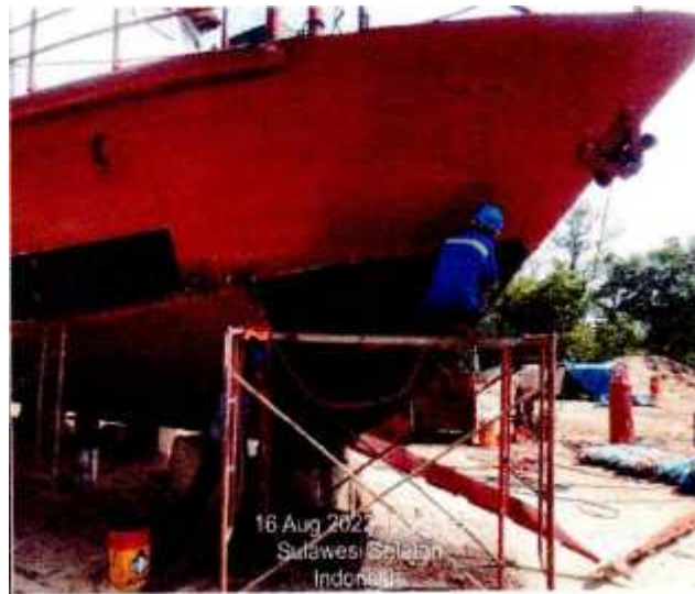
Gambar 12 Proses Cropping Lambung Haluan Kanan
