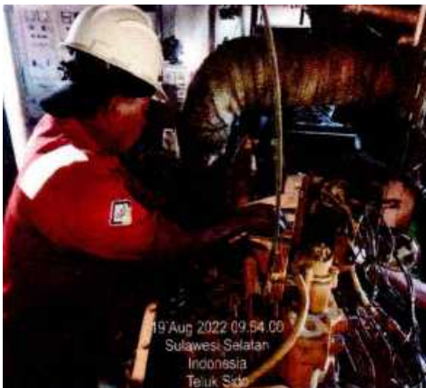
Gambar 18 Top Overhaul Main Engine Kiri
