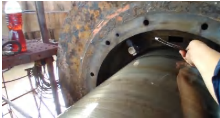
Pengukuran clearance as propeller
