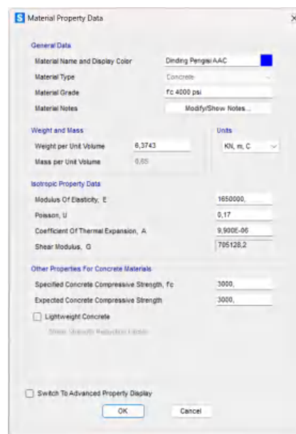
Gambar 6. Tampilan Material Concrete (dinding pengisi)
