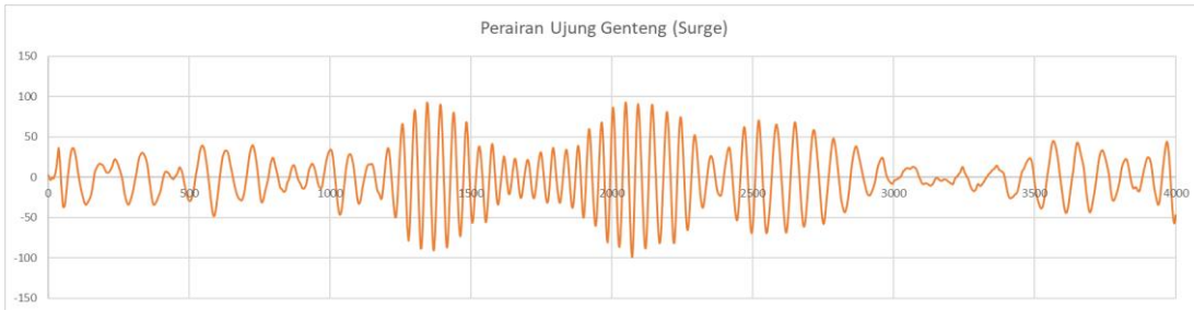
Lampiran 14. Grafik hasil running structure position surge, sway, heave, roll, pitch, dan yaw MIT/NREL TLP 5MW pada Perairan Ujung Genteng
