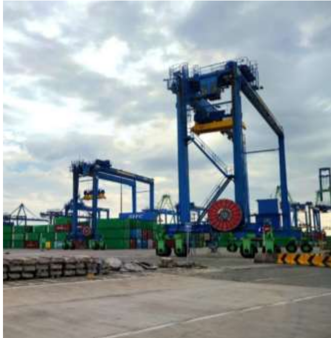
Gambar 2.1 Rubber Tyred Gantry Crane TPK New Makassar 2
