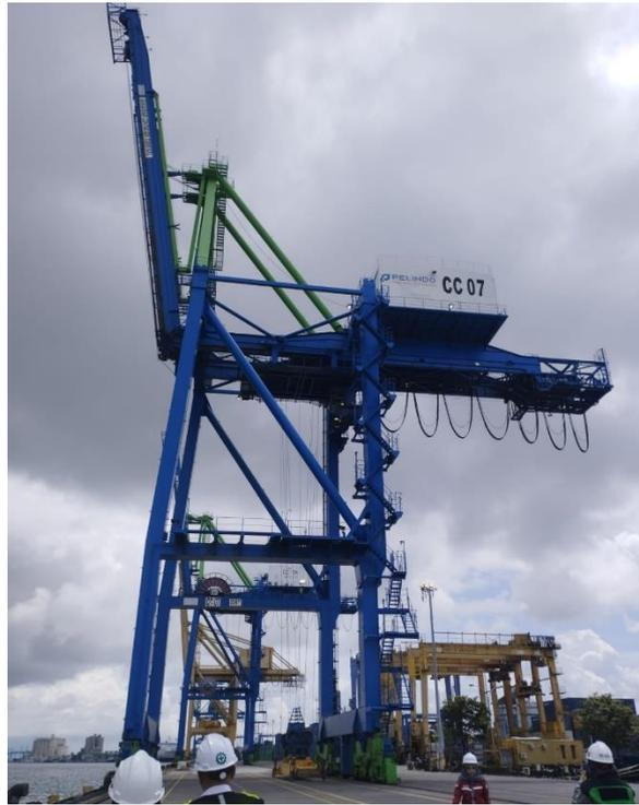
**Gambar 2.2** *Ship to Shore Container Crane*
