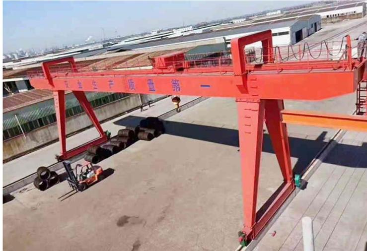
**Gambar 2.4** *Rail Mounted Gantry Crane (RMGC)*
