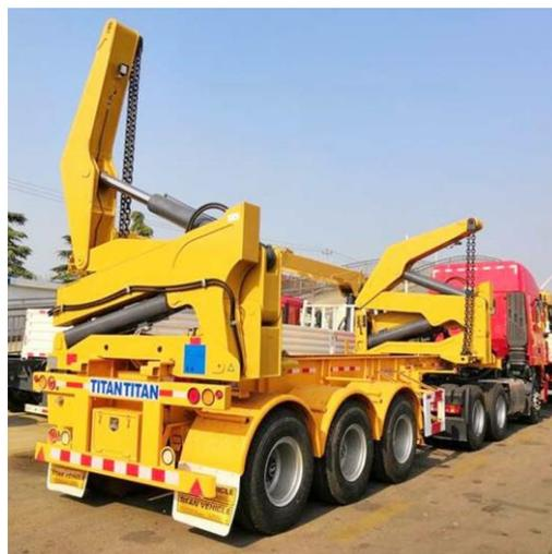
**Gambar 2.9 Side Container Loader**
