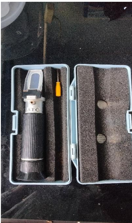
Lampiran 7. Alat Pengukur Salinitas Air (Refractometer)
