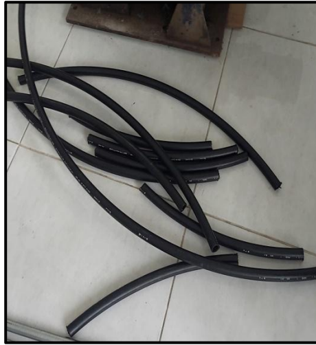
Gambar 42 Pipa high density polyethylene (HDPE)
