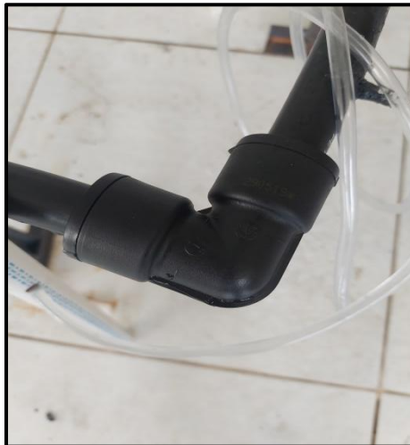
Gambar 33 Elbow 90° hdpe ¾ inch
