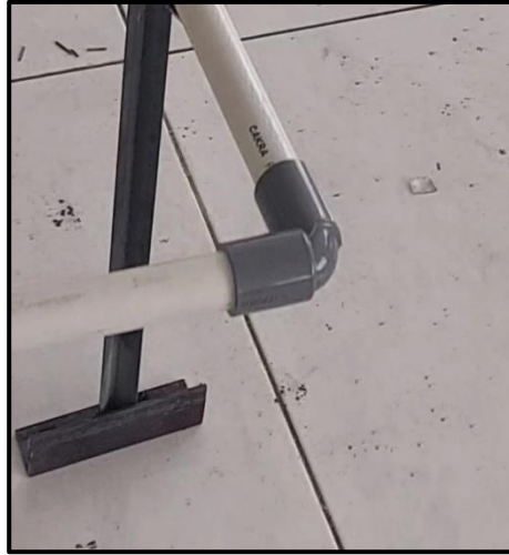
Gambar 32 Elbow 90° pvc ¾ inch
