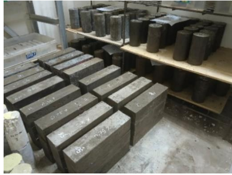
Lampiran 6. Proses curing udara beton geopolimer
