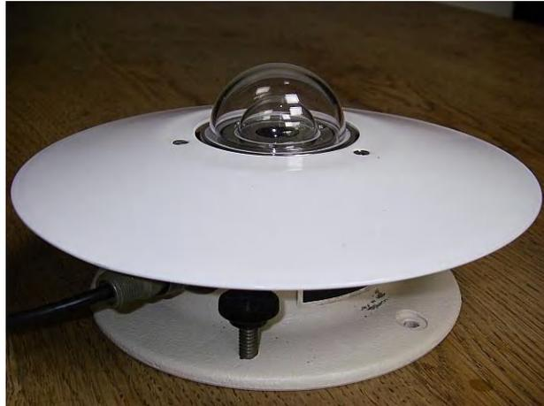
Gambar 2.15. Pyranometer PSP Eppley
