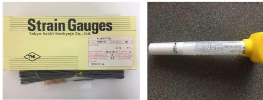
(a) Strain gauge beton
