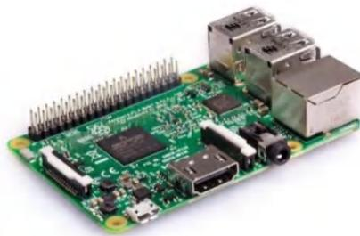
Gambar 3. *Raspberry Pi 3 Model B*
