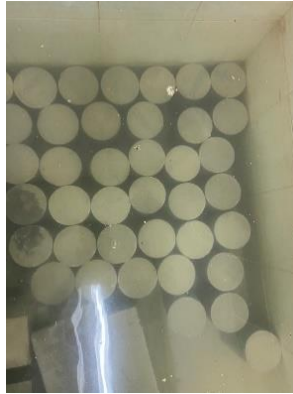
Curing Benda Uji
