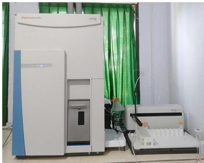
**Gambar 3.** Instrumen ICP-MS
