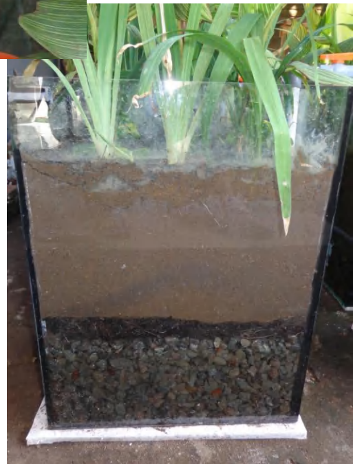
Gambar 13 Reaktor Constructed Wetland
