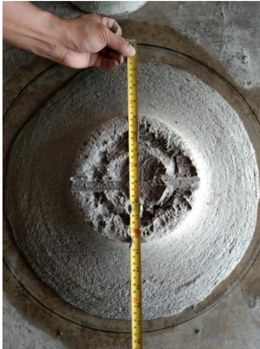
Gambar 22. Uji Slump Flow Beton Busa
