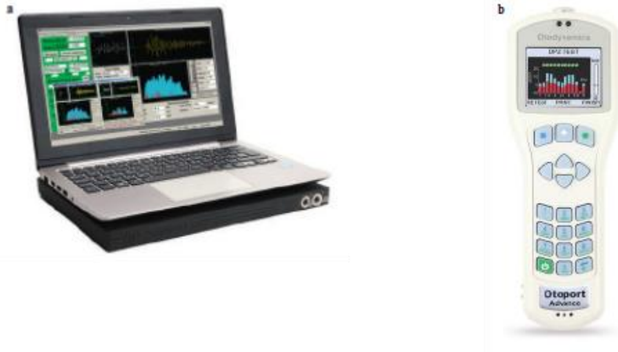
Gambar 17. Instrumen OAEs, a. tipe desktop; b. tipe hand-held.
