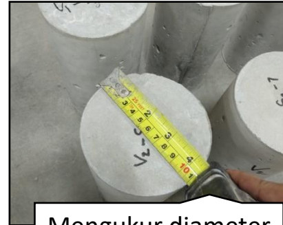
Mengukur diameter beton
