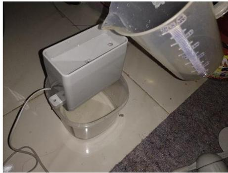
Gambar 2. 8 Kalibrasi Sensor *Rain Gauge*
