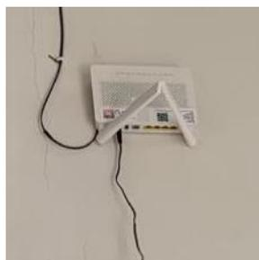
Gambar 7 ONT (*Optical Network Terminal*) (PT. Biznet)
