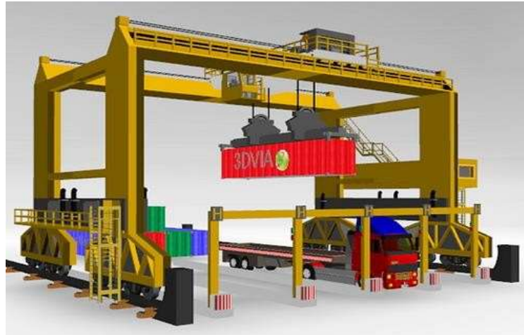
Gambar 5. Rail Mounted Gantry Crane (RMGC)
