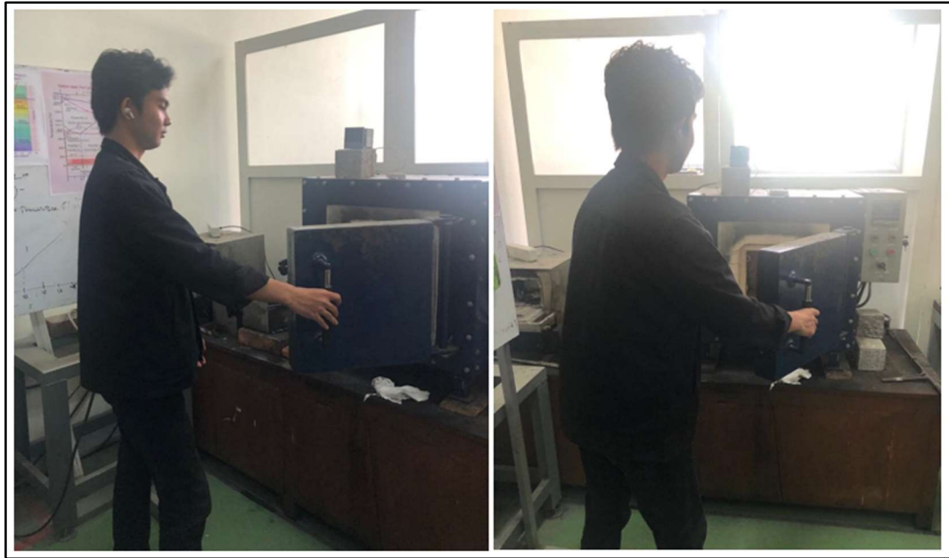
Gambar C.1 Proses Heat treatment perlakuan annealing batang tembaga
