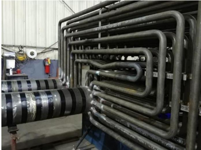
Gambar 3 Pipa Superheater
