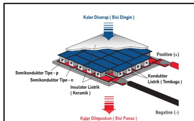
Gambar 1 Cara kerja Thermoelectric [11].
