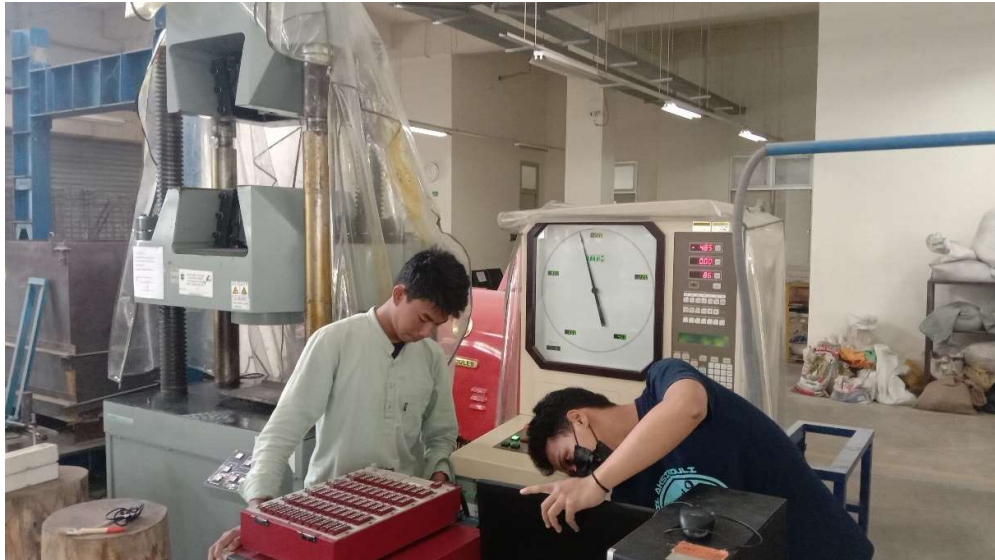
Set Up Alat Pengujian Pull Out
