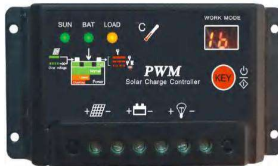
Gambar 2.10 Solar Charger Controller
