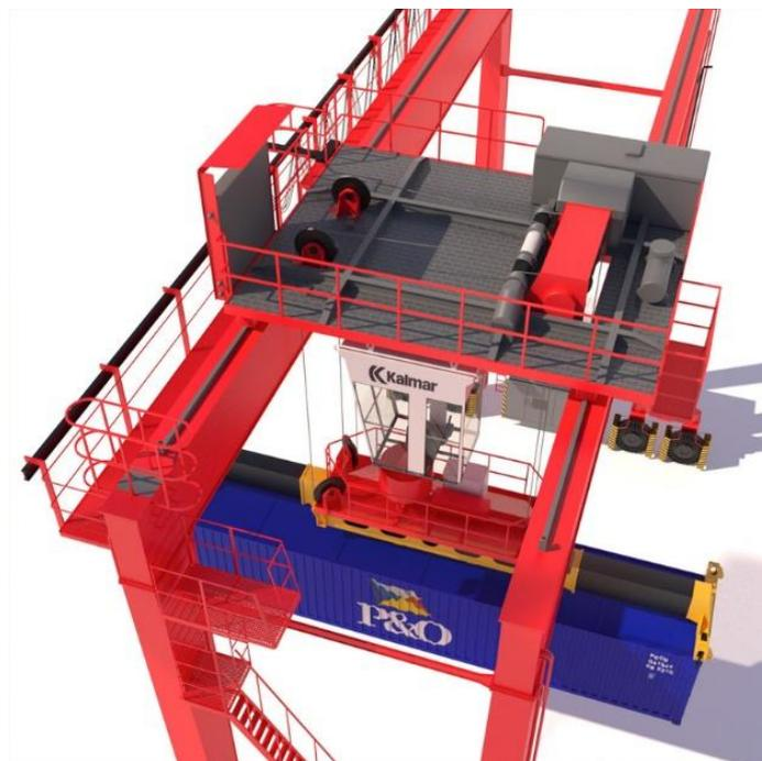
**Gambar 2.4** Trolley RTG Crane
