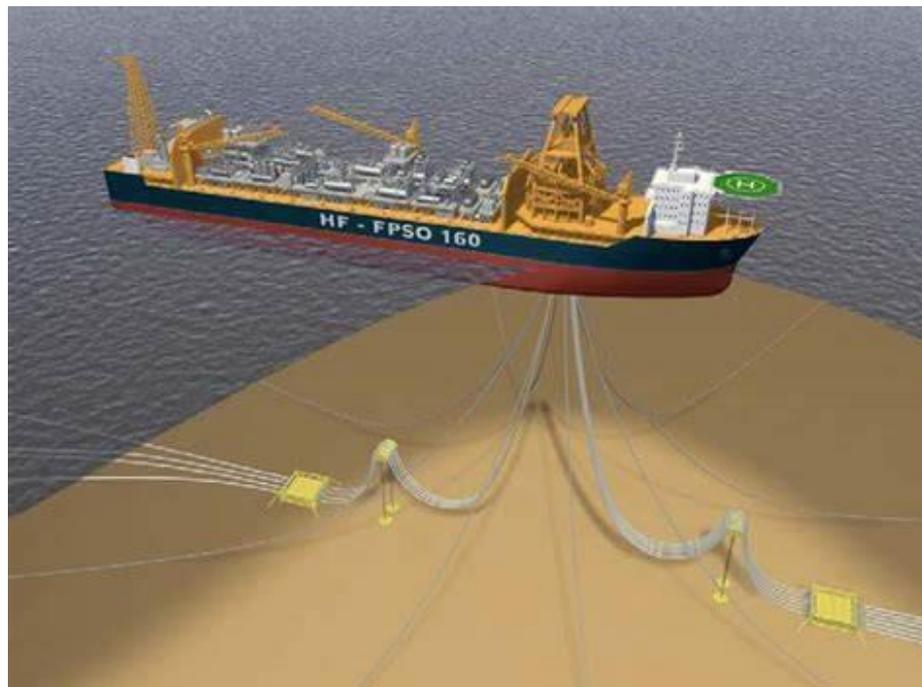
**Gambar 2.1** *Floating Production Storage and Offloading (FPSO)*
