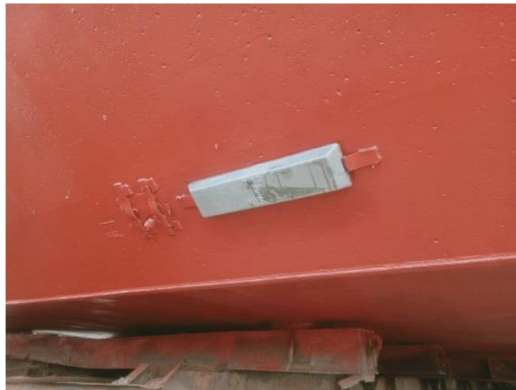
Gambar 2.9 Longated flush-mounted zinc anode
